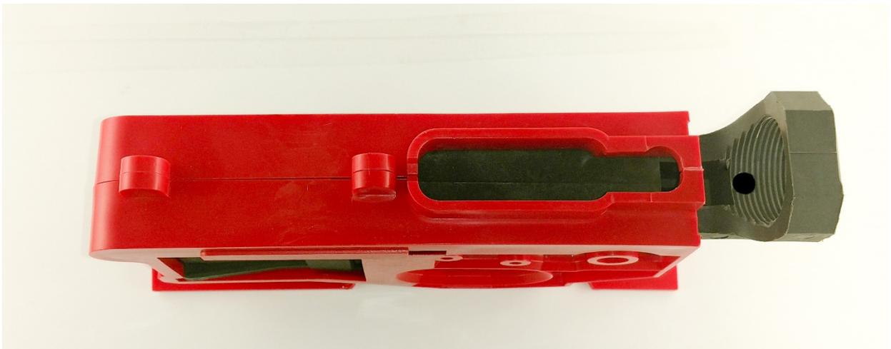
**Top View with Lower Receiver inserted into Jig**
