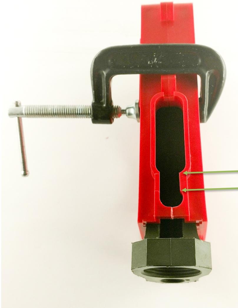
Note how the area of the jig that is **off-centered slightly (where the green arrows are pointing)**. Below this area is where the safety selector detent and spring hole come in from underneath the receiver where the pistol grip is attached. This area is extremely close to the edge where you will be milling.
